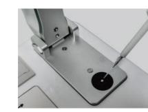
Suck 0.5~2.0uL sample buffer onto the testing machine base, lower the testing arm, click "blank" to obtain the baseline, and wipe it clean with dustfree paper after completion Colorimetric dish detection.
