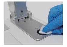
After testing, use 0.5~2.0uL clean two sample holders and two light holders with ultrapure water, and wipe the solution clean with dust-free paper; 3 to 4 times.
