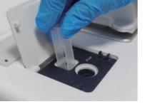
Insert the OD600 detection cuvette solt and click on "sample" to test the absorbance of the sample.
