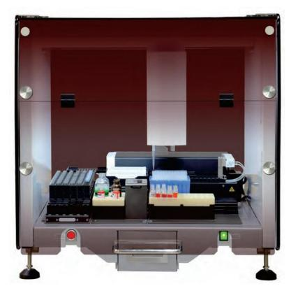
URANUS AE 55 is a dedicated system to automate microplate-based ELISA tests and deliver accurate results with high efficiency. adopting the modular automation concept, URANUS AE 55 equips with liquid handing module, incubation module, plate washing module, microplate readers, flexible mechanical grippers to transfer microplates between modules, an intelligent software control.
