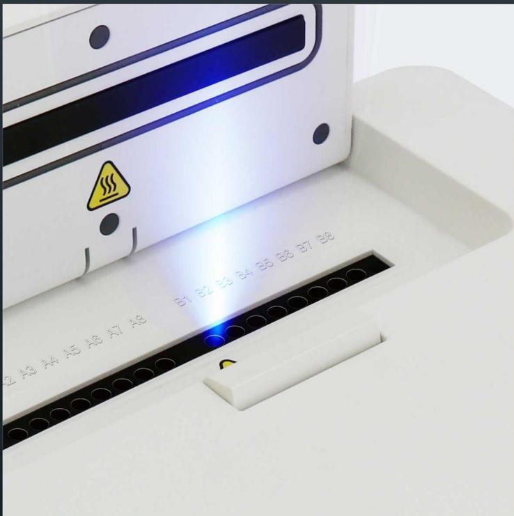
In UV scan (hot lid should be closed in actual work)
